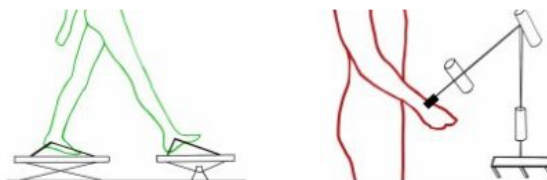
Figure 1-1: Illustrations of end-effector robotic devices, lower limb (left) and upper limb (right). Source: [3]
